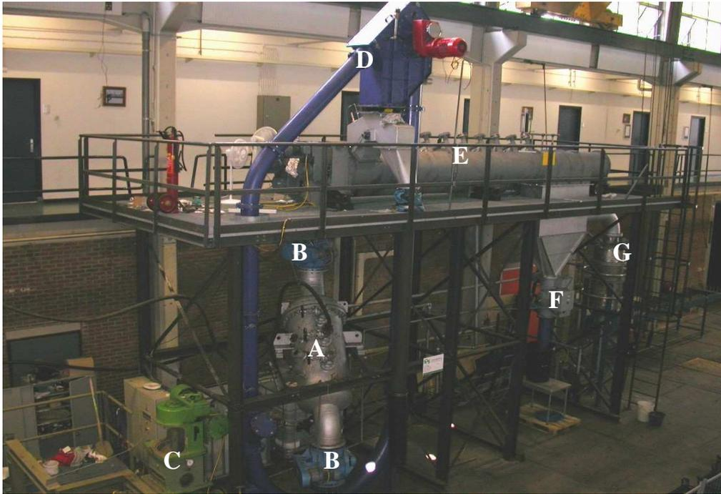
**Figure 3: The prototype consists of a steam vessel (A), two rotary sluices (B), an extruder (C), an elevator (tube chain conveyor) (D), two screw conveyors (E), a vacuum sluice (F), a condenser (G), a vacuum pump, and a water pump. Except from the screw conveyors, these are all more or less standard components.**
