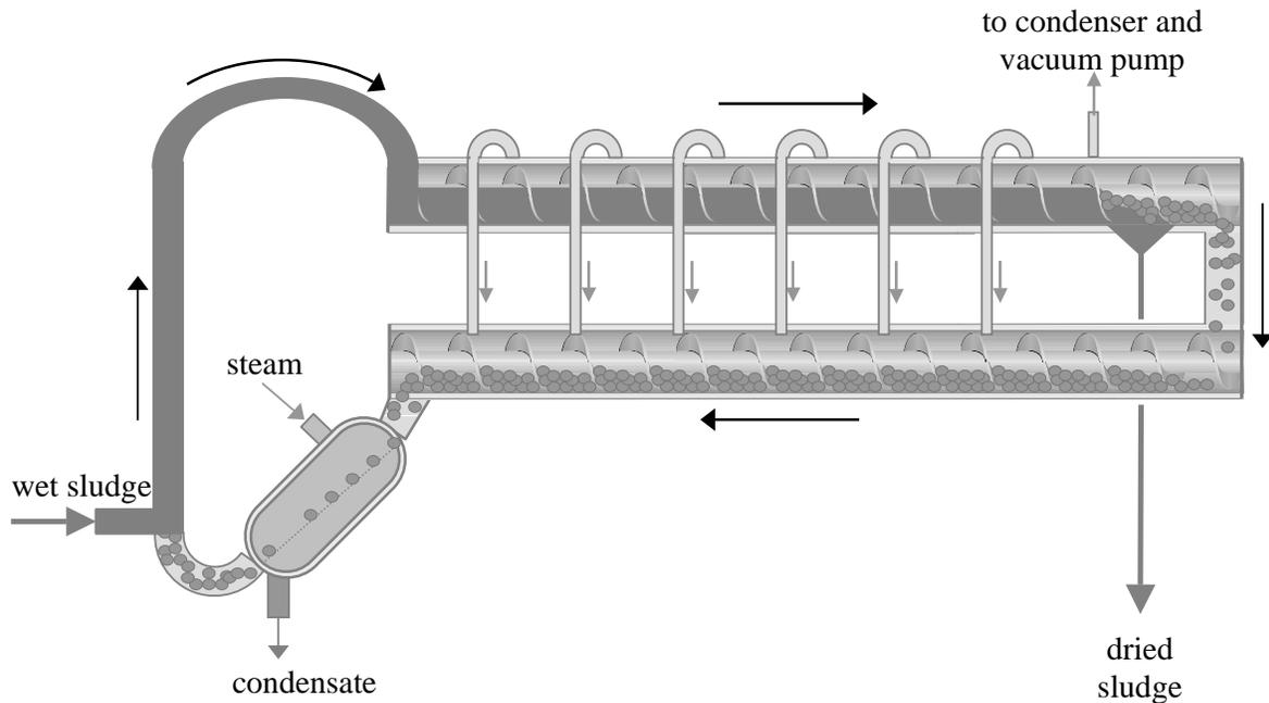
**Figure 2: Schematic representation of the Delta dryer, showing a closed circuit of metal balls. At the left side the balls are mixed with wet sludge. In the upper conveyor the mixture dries up and cools off, whereas cooler return balls are stepwise reheated by sludge vapour in the lower conveyor. At the end of the lower conveyor the partially reheated balls are fed into steam vessel.**
