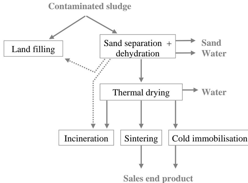
**Figure 1: Different processing routes for contaminated sludge.**
