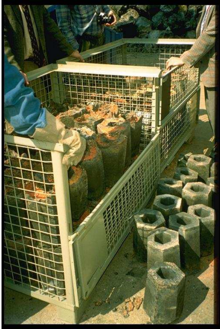
Figure 2. Basalt made out of dredging spoil
